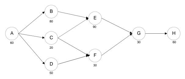
b. What is the workstation cycle time required to produce 240 units per day?
