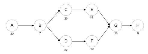
d. Balance the line using sequential restrictions and the longest-operating-time rule.
