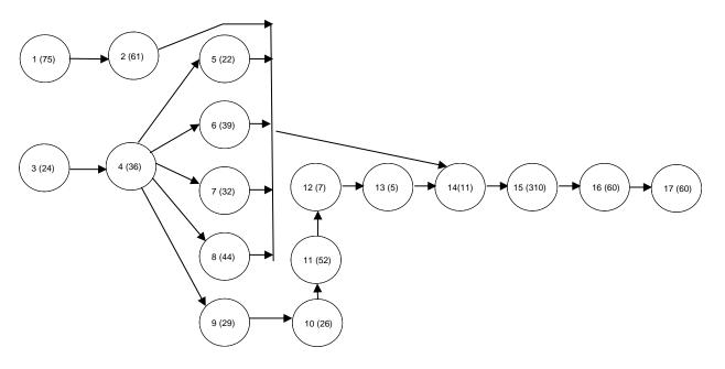
This may be possible with a redesigned line, but we might not have enough line positions to accommodate the new design. The following is a design that was constructed using the "longest task" priority run. This is actually a pretty good design and it would be possible to make 300 units per day. The labor efficiency of this line is 583/(8(90)) = .809 or 81%. [Since stations 7-9 are not staffed, they are not included in the efficiency calculation.]
