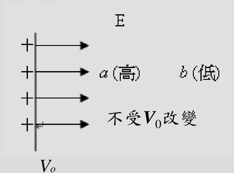
$$\left\{ \begin{array}{l} V_a - V_0 = -E \cdot (a - 0) \\ V_a = V_0 - E \times a \\ V_b = V_0 - E \times b \end{array} \right.$$
