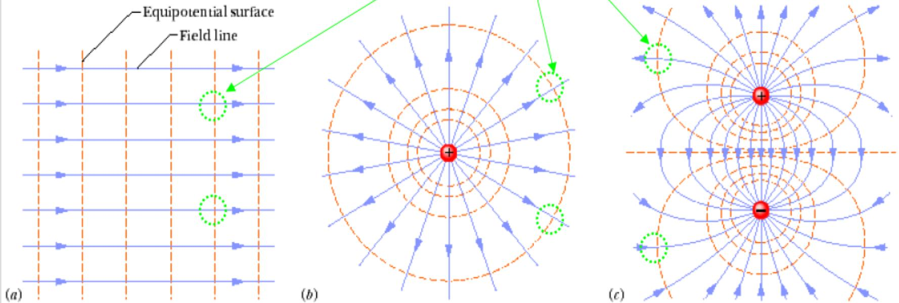
**Fig. 24-3** Electric field lines (purple) and cross sections of equipotential surfaces (gold) for (a) a uniform electric field, (b) the field due to a point charge, and (c) the field due to an electric dipole.
