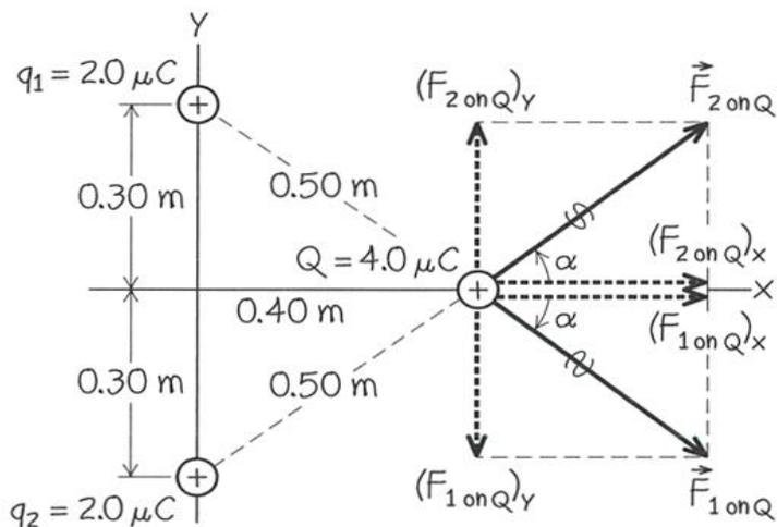
**EXECUTE:** Figure 21.14 shows the forces  $\vec{F}_{1 \text{ on } Q}$  and  $\vec{F}_{2 \text{ on } Q}$  due to the identical charges  $q_1$  and  $q_2$ , which are at equal distances from  $Q$ . From Coulomb's law, *both* forces have magnitude
